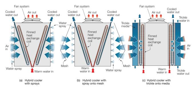
Figure 1.4 Dry/wet cooling systems
