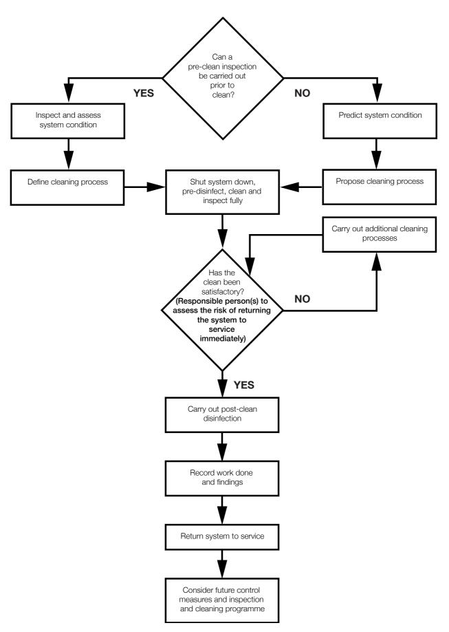
Figure 1.7 Flowchart of inspection and cleaning decision-making process
