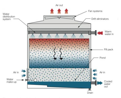
Figure 1.1 Induced draught counterflow cooling tower
